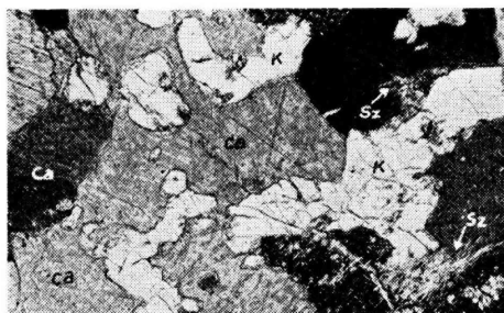
Fig. 12. Photomicrograph of Kotoite-marble from Rézbanya, Romania ( \times 90 , crossed nicols). K: Kotoite Ca: Calcite Sz: Szaibelyite
